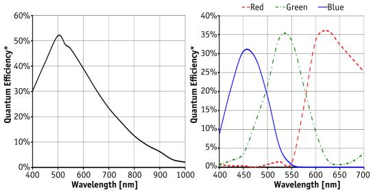
\*QE measured without protection glass or filters. With glass or filters, quantum efficiency decreases by approximately 10%.
