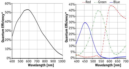
\*QE measured without protection glass or filters. With glass or filters, quantum efficiency decreases by approximately 10%.
